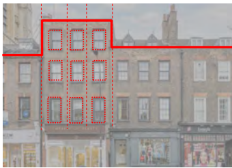
Traditional Brick Terraces to Kensington Church Street: Punched hole and facade rhythm & Stepped Roofscape
