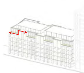
4. Articulated frontage to break continuous parapet line
