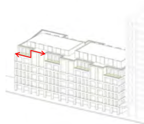
4. Articulated frontage to break continuous parapet line
