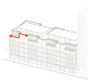
4. Articulated frontage to break continuous parapet line
