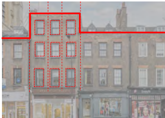
Traditional Brick Terraces to Kensington Church Street: Punched hole & Stepped Roofscape
